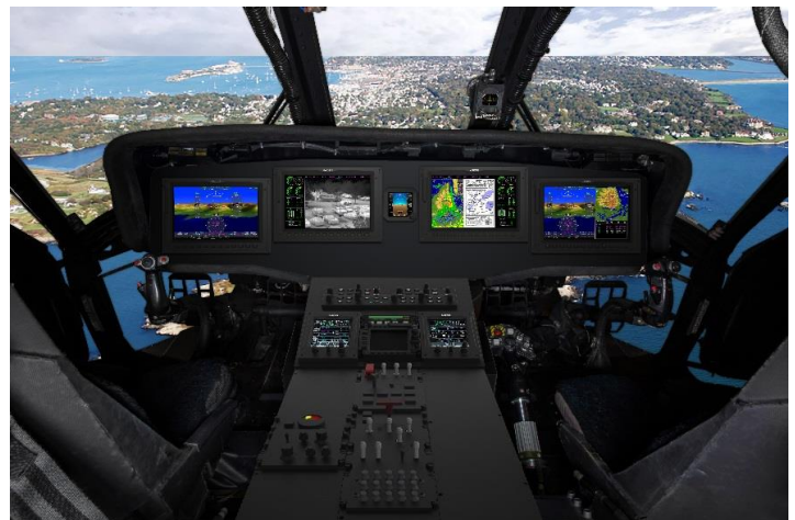
ACEHAWK Cockpit with Garmin® G-5000H and Avalex Cockpit Management Unit
